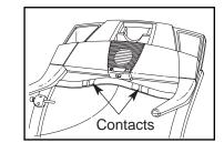
sensor with your palms resting on the metal contacts. **Avoid moving your hands**. When your pulse is detected, two dashes (– –) will appear in the Calories/Pulse display, and then your heart rate will be shown. **For the most accurate heart rate reading, continue to hold the contacts for about 15 seconds**.
